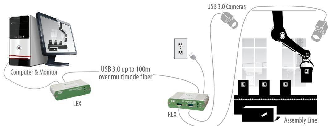
\* Up to 50m with USB 3.0 storage type devices; up to 100m or more is achievable when using USB 3.0 bulk traffic cameras. For Microsoft Kinect applications, please use the Spectra™ 3001-15 active extension cable.
