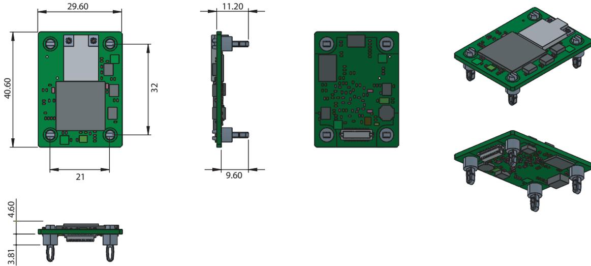
**Panel Cut-out Dimensions: 40.6mm x 29.6mm x 14.2mm**
