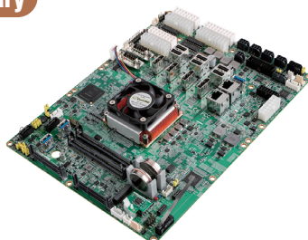
DPX-E145 board with active cooler
